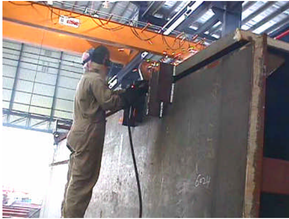
Figure 14. Semi-automatic welding of spine beam.
